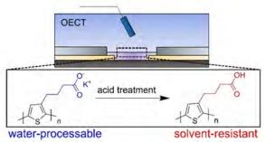
Water-soluble precursors can be spray cast on transistor substrates and acidified to yield solventresistant materials with substantial electroactivity in aqueous and organic media.
